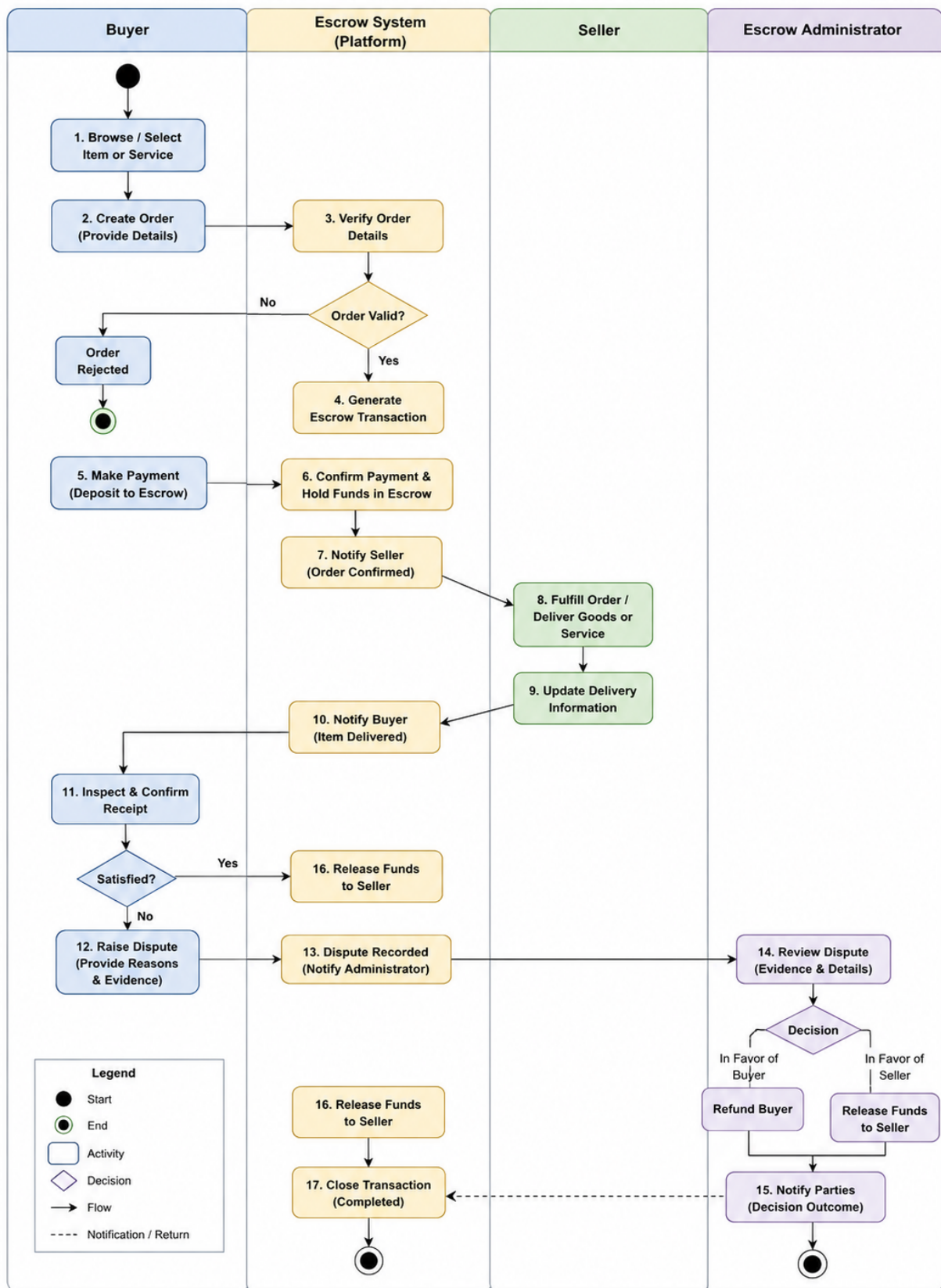
Figure 6. Activity Diagram of the Escrow Transaction Workflow.
