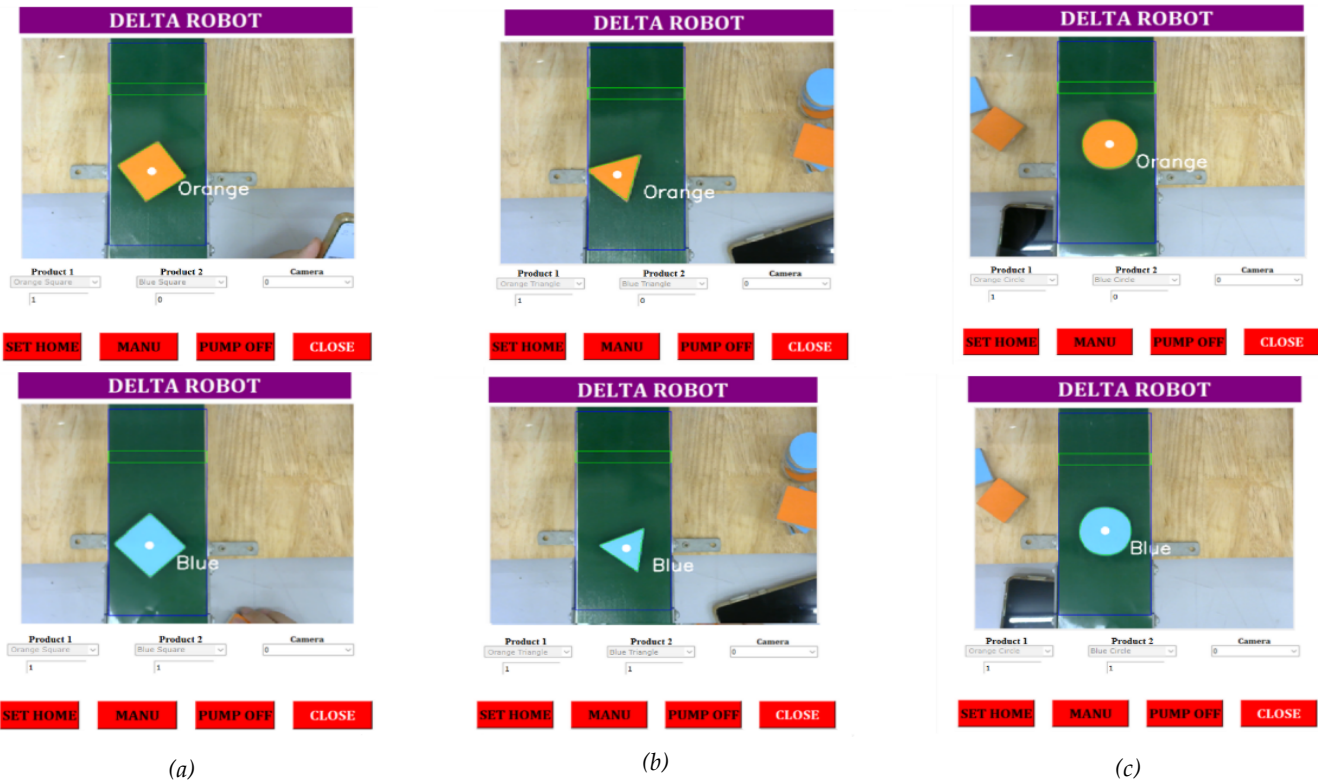
Figure 8. Image processing results, for (a). square objects, (b). triangle objects, and (c). circle objects.
