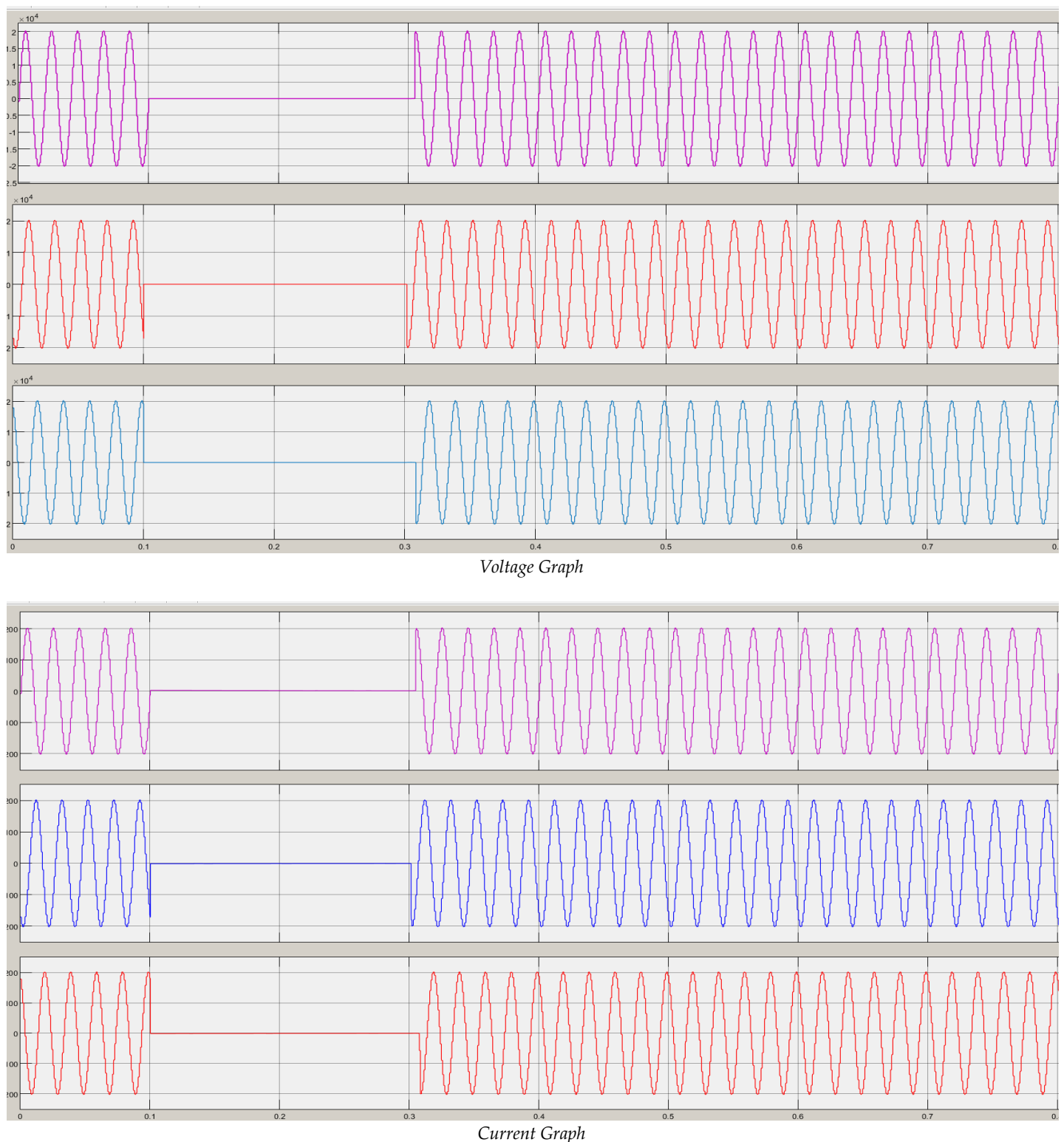
Figure 8. Simulation Output (Time delay Protection).
