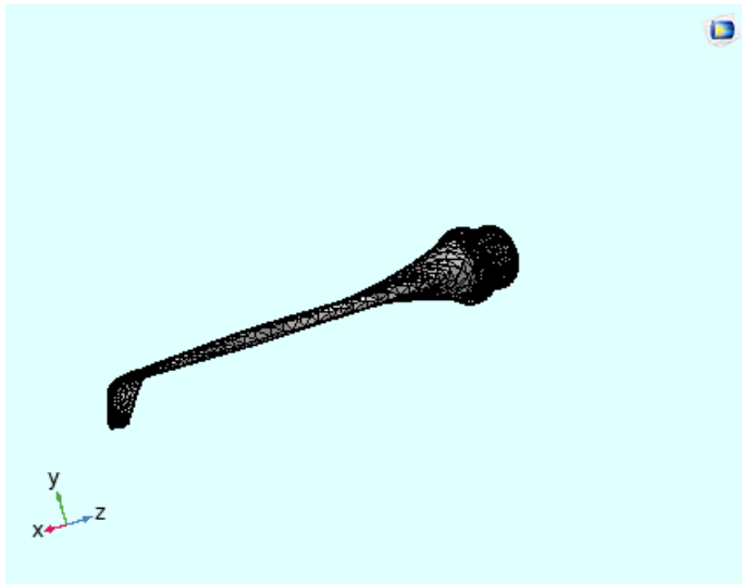
Figure 2. Meshing configuration around the blade.
