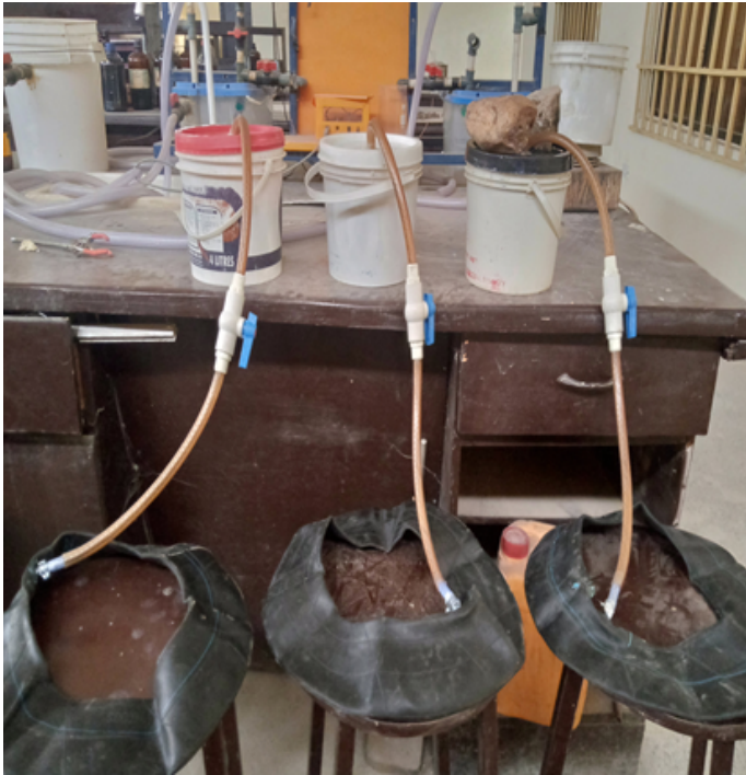
Figure 2. Biogas Production Setup for Bioaugmentation.
